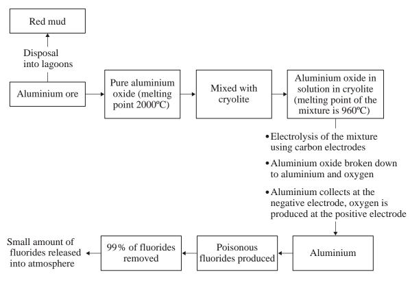
(a) The red mud from the aluminium ore is disposed of by dumping in lagoons. The red mud contains iron oxide.
