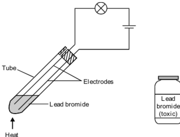
Lead bromide was placed in the tube and the circuit was switched on. The light bulb did not light up.
