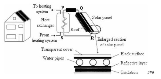
A The different layers of the solar panel make the panel transfer solar energy in the most effective way. Which row of the table shows how each layer helps this?
