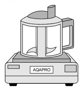
The food processor is designed to transfer electrical energy to kinetic energy. However some of the energy is wasted as heat and sound.
